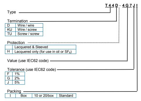
Note: Standard TCR is 100ppm/°C. Contact factory for 50 and 25ppm/°C grades.
